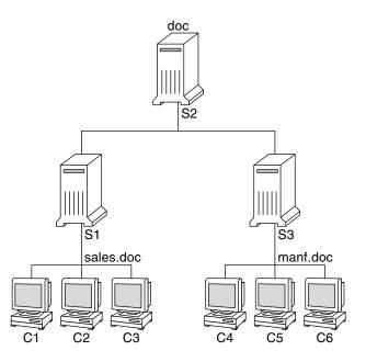
Clients C1, C2, and C3 would obtain their network information from server S1. Clients C4, C5, and C6 would obtain information from server S3. The resulting network is summarized in the following table. The table is a generalized representation of that network but does not resemble an actual network information map.
