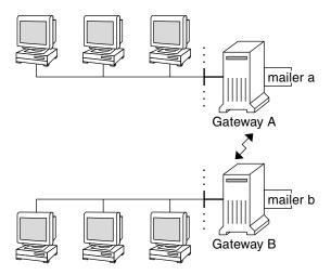
FIGURE 14–1 Gateway Between Different Communications Protocols
