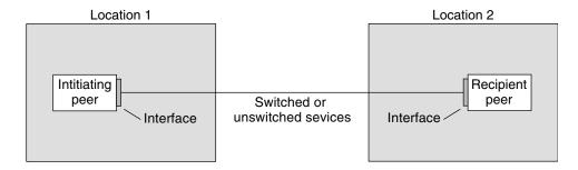
FIGURE 15-1 Parts of the PPP Link
