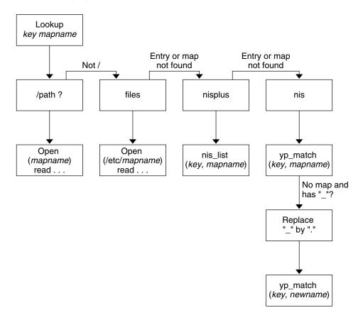
FIGURE 6–6 How Autofs Uses the Name Service
