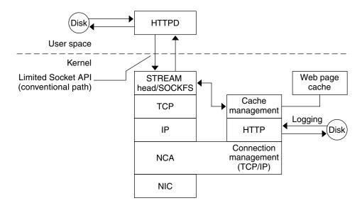
FIGURE 2-1 Data Flow With the NCA Service
