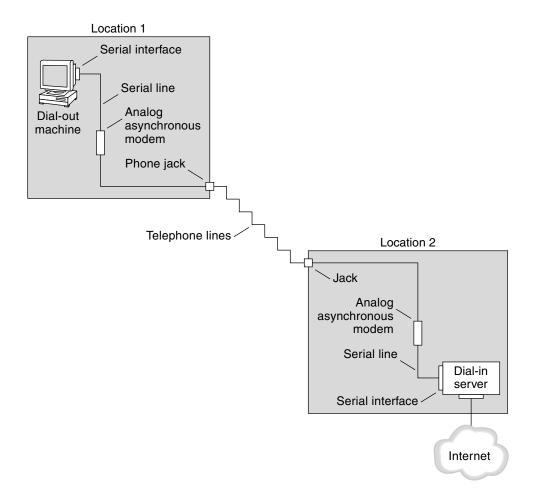
FIGURE 15-2 Basic Analog Dial-up PPP Link
