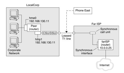
FIGURE 16-2 Example of a Leased-Line Configuration
