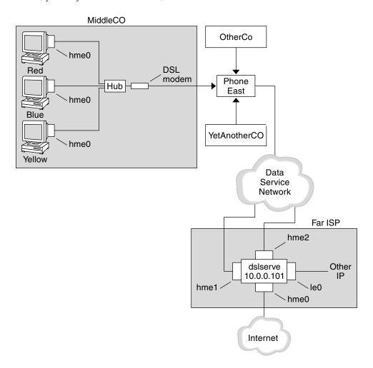
FIGURE 16-5 Example of a PPPoE Tunnel
